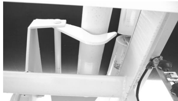
Hanging Weight on Weigh-bridge
