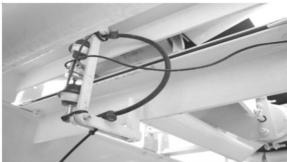
Weigh Bridge Load Cell
